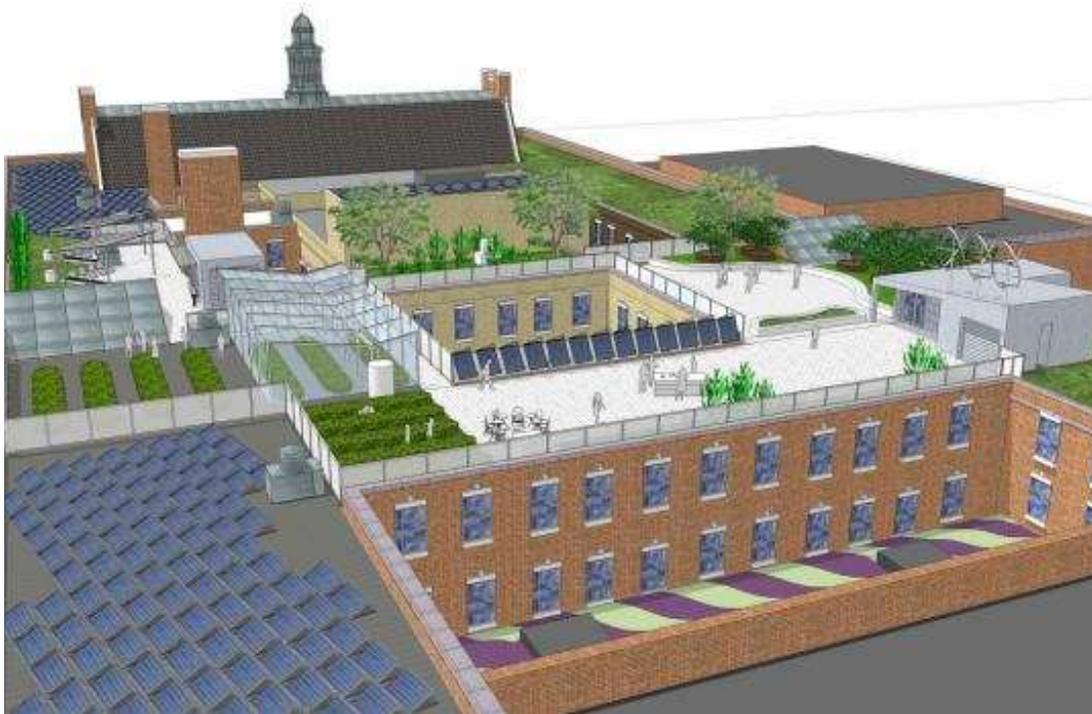
**An artist's rendering of the Boston Latin School's green roof shows a new stairway and elevator, as well as a greenhouse and cafeteria. The greenhouse will be heated by solar thermal panels. (Studio G Architects)**
